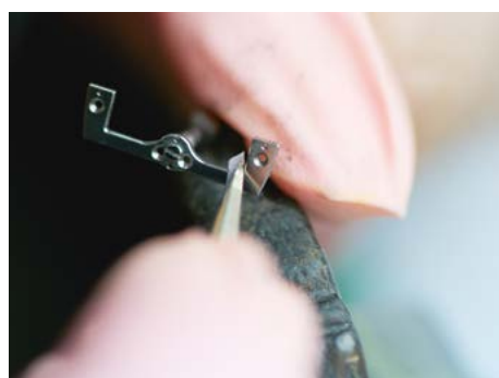
4 The beveling is made with a tool called “carbon”, but we often have to make the exact tool we need ourselves. We sometimes break a metal tweezers in 2 and we glue the abrasive paper on one of the half.
