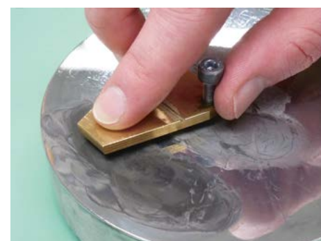
8 Mirror polishing, also called “black polish”, is performed on a zinc plate with polishing paste prepared in house. The component is polished this time in a circular gesture.
