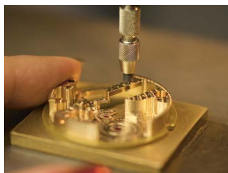
3 The perlage by hand is a succession of superimposed circles, resembling pearls, which requires a great dexterity and an adapted rhythm for the regularity and density of the pearls.
