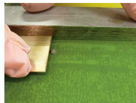
7 The operation for “traits tirés” is done on a zinc plate with polishing paste. The gesture is straight from top to bottom and repeated until they are perfect.
