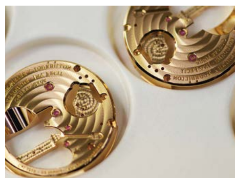
6 Côtes de Genève are performed on a semi-automatic machine that need numerous settings before starting this operation.
