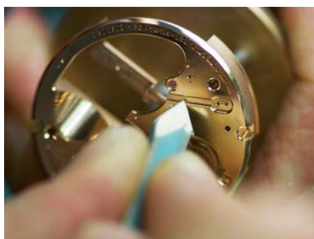
1 Finishing of angles with a “cabron” (wooden stick covered with sand paper) before polishing.
