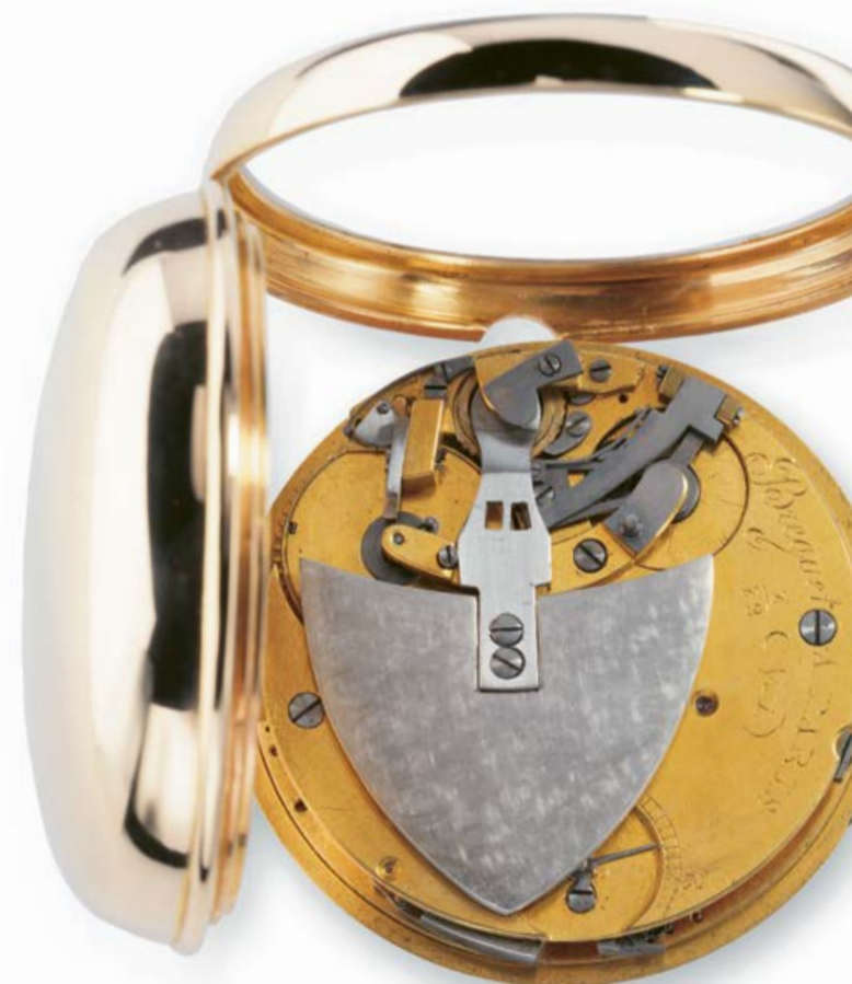
Breguet watch with quarter repeater N° 28 circa 1784, with gold helmet-shaped winding weight, pivoting on the edge of the back plate, signed Breguet à Paris, Patek Philippe Museum, Geneva.
