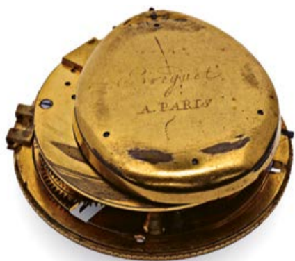
Movement signed Breguet à Paris. View of the back plate and the striking work of the movement.
