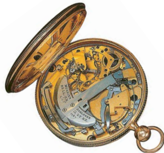
Self-winding watch by Charles Mugnier N° 1167 in gold made for Napoléon 1 st with quarter repeater, small second and oscillating mass sunken into the movement.
