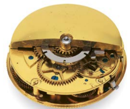
Movement of one of the few self-winding watches assignable to Perrelet. The weight pivoted in the centre oscillates with no limitation of amplitude. Patek Philippe Museum, Geneva.
