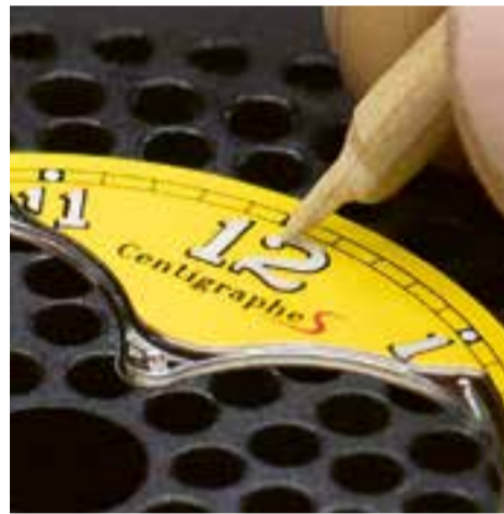
Positioning of a luminescent numeral on the dial of the Centigraphe.
