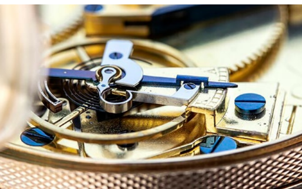
“Parachute” system Invention of Abraham-Louis Breguet in 1790, featured on a subscription watch. © The Naked Watchmaker.
