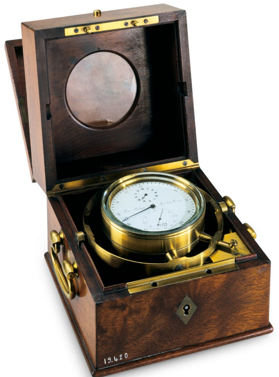
Marine chronometer No. 159, by Louis Berthoud © Musée des arts et métiers, Cnam. Photo by Sylvain Pelly.
