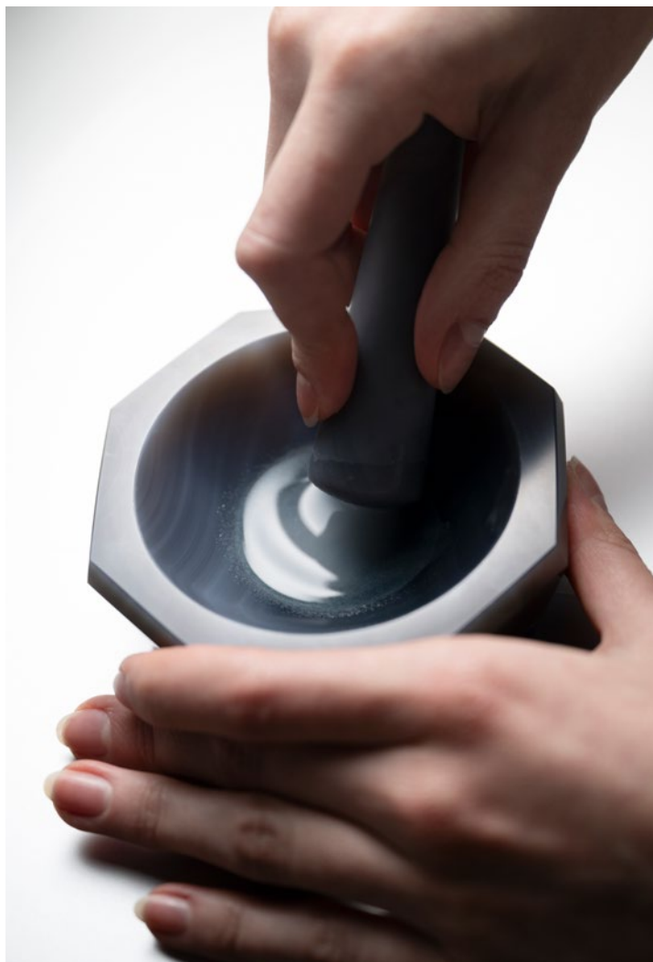
Preparation of the enamel: The enamel is finely ground in a mortar with water to create a homogeneous paste, ready for application.
